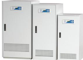
XT Series Online UPS are microprocessor controlled, full sine output uninterruptible power supplies produced with PWM (Pulse width modulation) and IGBT technologies. It provides uninterrupted energy for local networks, communication systems, sensitive medical devices, smart engineering measuring devices and industrial automation systems by guaranteeing safe operation thanks to its built-in inverter isolation transformer.
