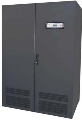
4000 Series 3 phase, 4 pole static transfer switch transfers uninterruptedly critical loads to either of two independent AC power lines. The system monitors two AC inputs. If any of them goes out of the specified tolerance, it transfers the critical load to the other. By increasing the energy quality of the systems used with 4000 Series, while reducing the effects of interference and short interruptions, a backup power system is gained.
