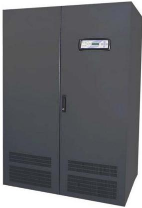
3000 Series 3 phase, 3 pole static transfer switch transfers uninterruptedly critical loads to either of two independent AC power lines. The system monitors two AC inputs. If any of them goes out of the specified tolerance, it transfers the critical load to the other. By increasing the energy quality of the systems used with 3000 Series, while reducing the effects of interference and short interruptions, a backup power system is gained.
